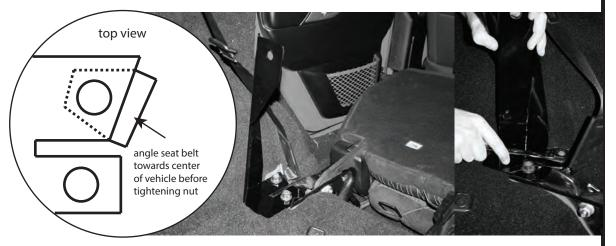
Factory Torque Spec: 62.5 ft/lbs rear seat mounting nut 30 ft/lbs seat belt bracket nut
